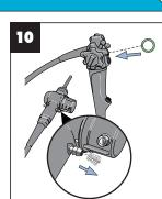
Brush the universal cord portion of the suction channel. Repeat until all debris is removed.
