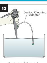
Aspirate detergent solution into suction channel.
