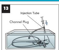
Attach injection tube and channel plug. Flush detergent solution into air, water and suction channels. Brush forcepselevator, if applicable.
