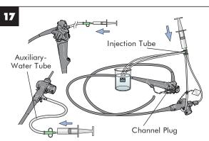
Flush clean water through all channels (including auxiliary-water/elevator-wire, if applicable). Flush air through all channels.
