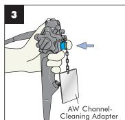
Install AW channelcleaning adapter. Flush water, then air, through air/water channels.
