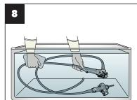
Immerse in freshly prepared detergent solution. Clean all external surfaces. Brush endoscope distal tip (and forceps-elevator, if applicable).
